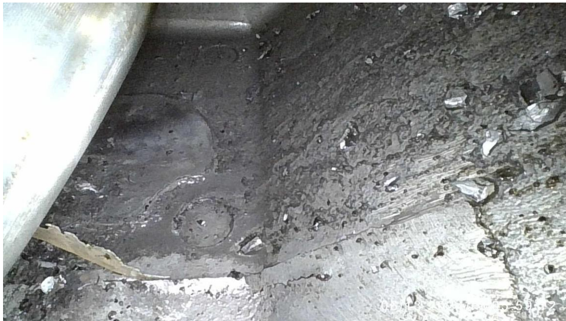
Figure 9. In sump. Not as much "Granola". Probably due to shutting down the engine quickly.
