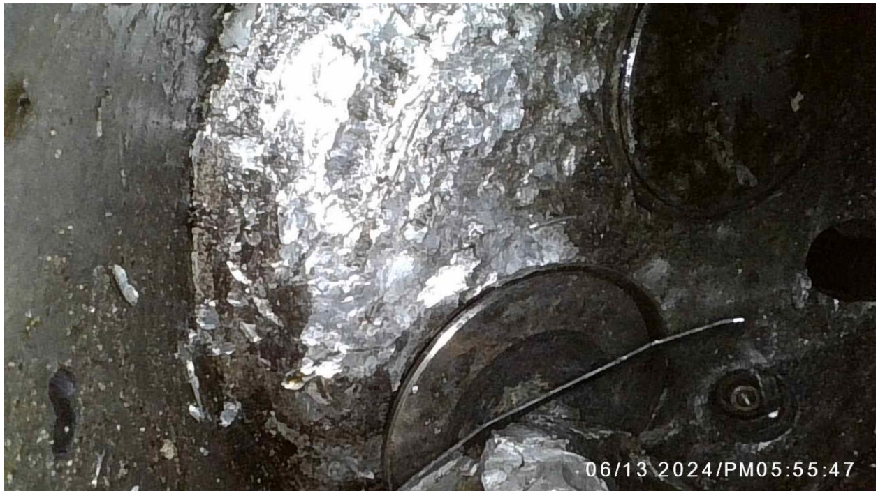
Figure 7. Both Valve are still in the head.
