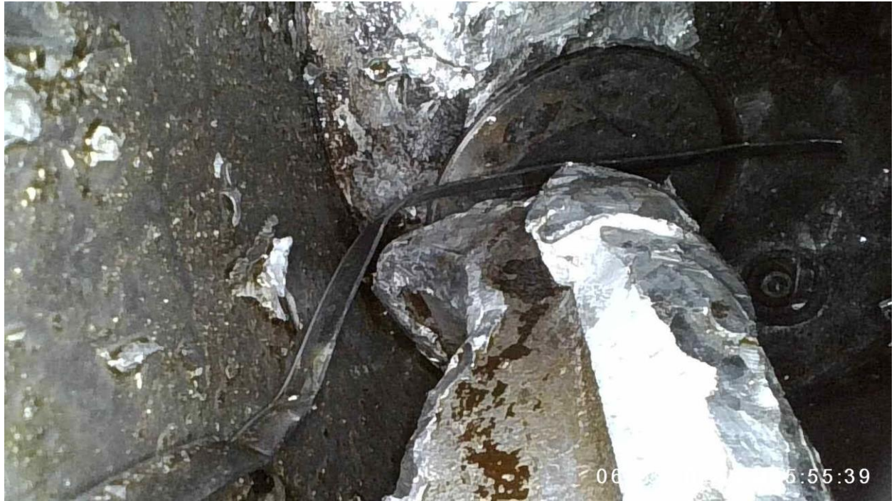
Figure 6. Valve with chunk of Piston
