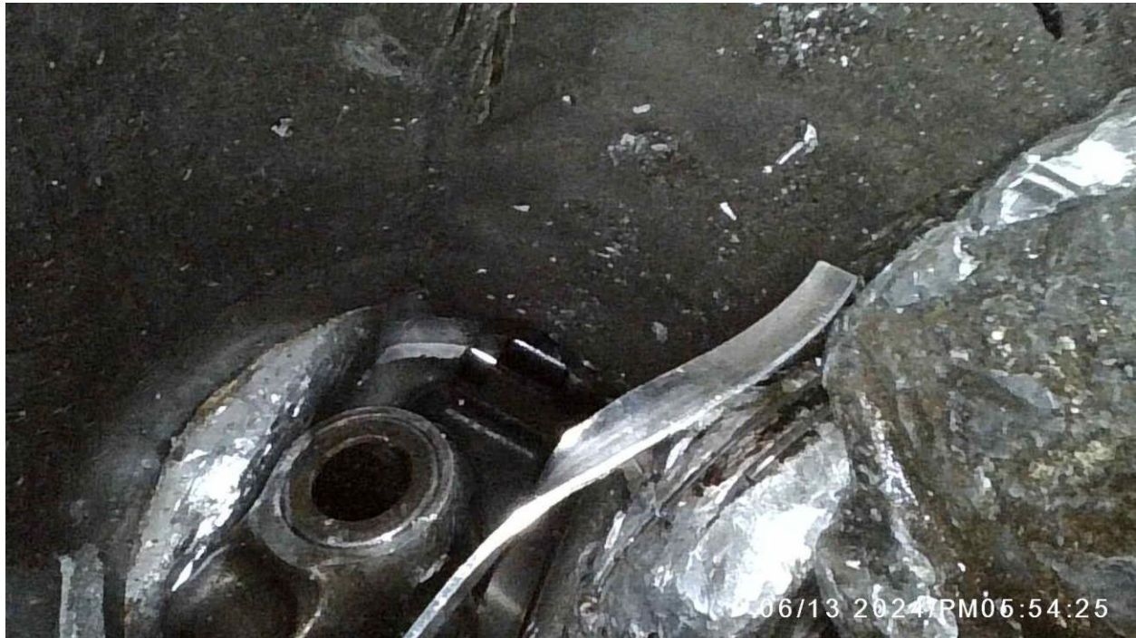
Figure 5. Bent over Rod and ring remains
