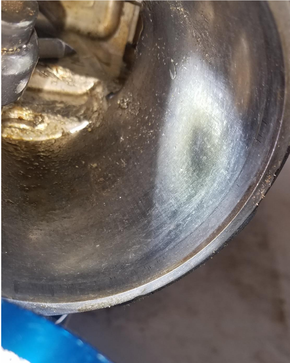
Figure 11. Picture of cylinder wall. Aside from the damage caused by the rod crushing the piston, the cylinder has no scratches, scoring or other damage.
