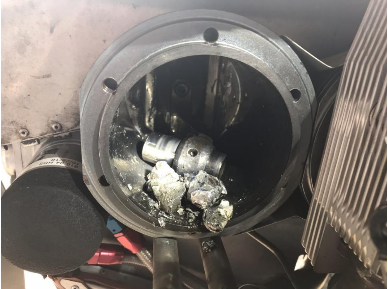
Figure 5. #2 Head removed. The piston is mostly missing, but the rod, wrist pin, and everything else is still there.
