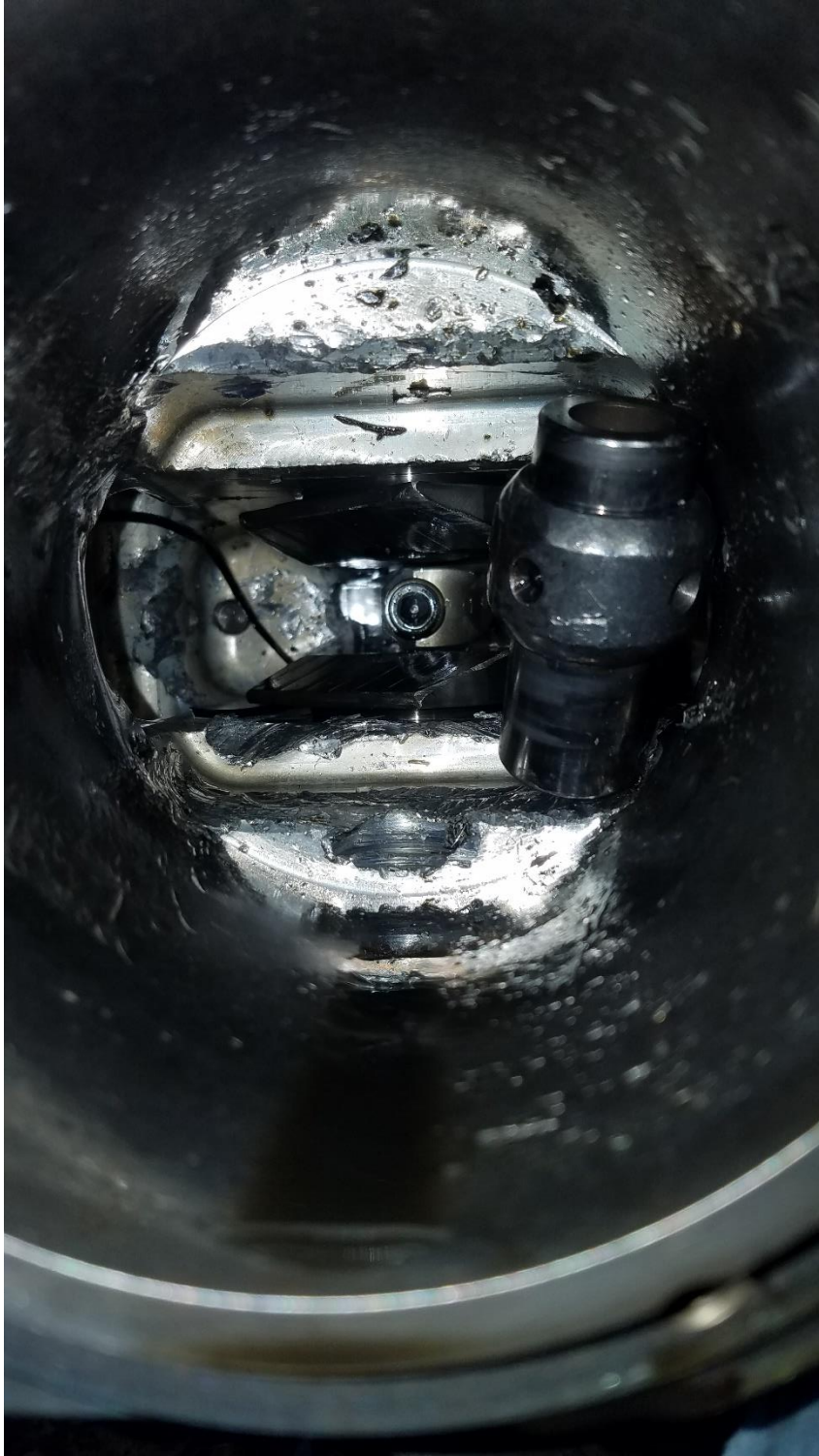
Figure 8. Inside the cylinder. Not including the damage caused by the rod/wrist pin beating against the cylinder walls, the cylinder looks actually quite good.
