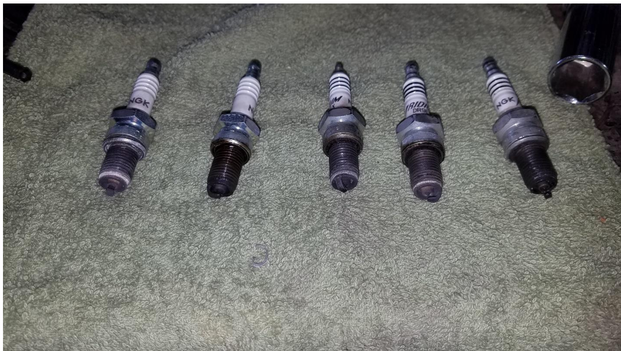
Figure 7. Spark plugs examined looking for signs of detonation. Cylinders were also borescoped for evidence, but none was found. Note that all plugs are black, indicating a rich mixture.
