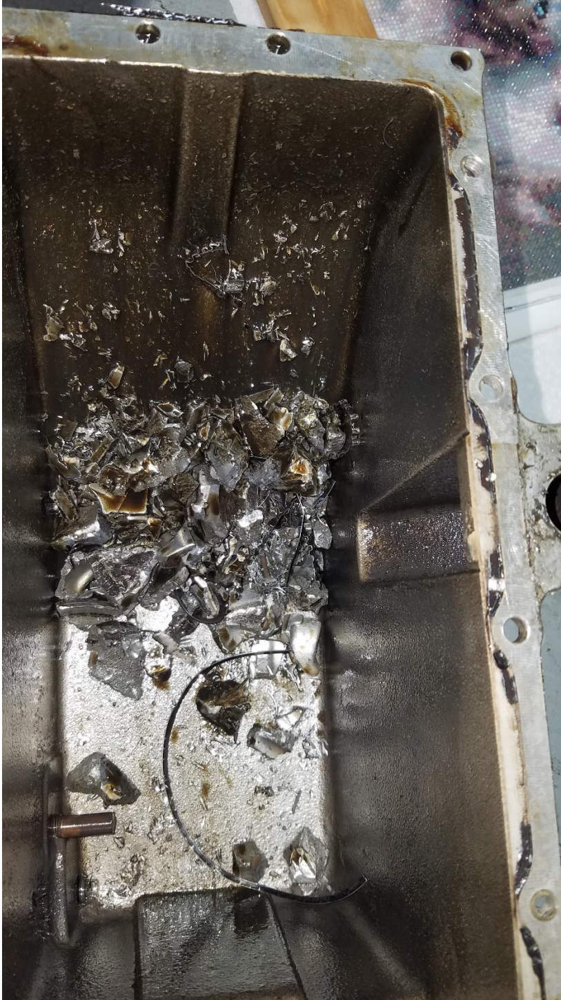
Figure 9. The rest of the piston, rings, and circlips were found in the sump.
