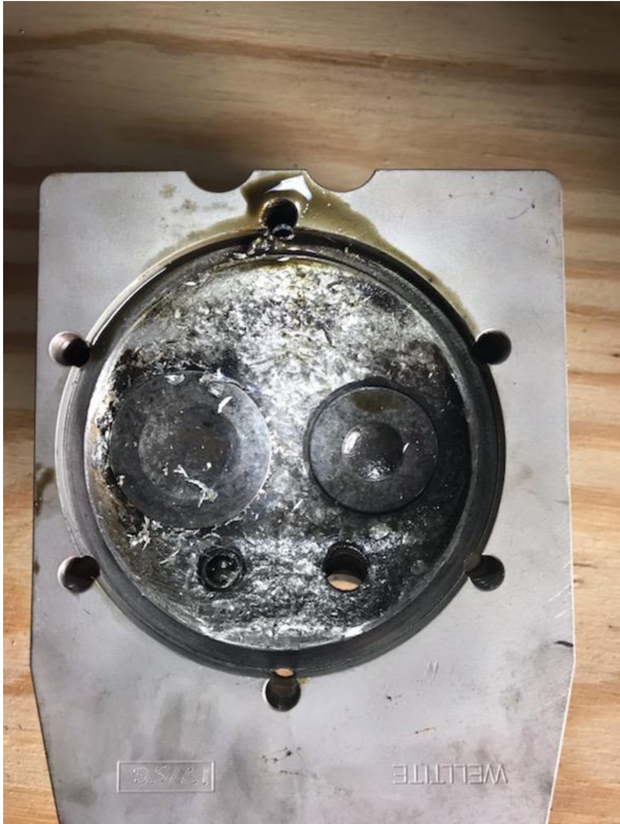
Figure 6. Head (cylinder face). Both valves remain. Exhaust valve has slight bend.
