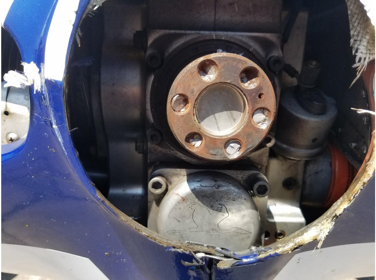
Figure 1. Note the missing prop hub and the fatigued screws still in the crankshaft.
