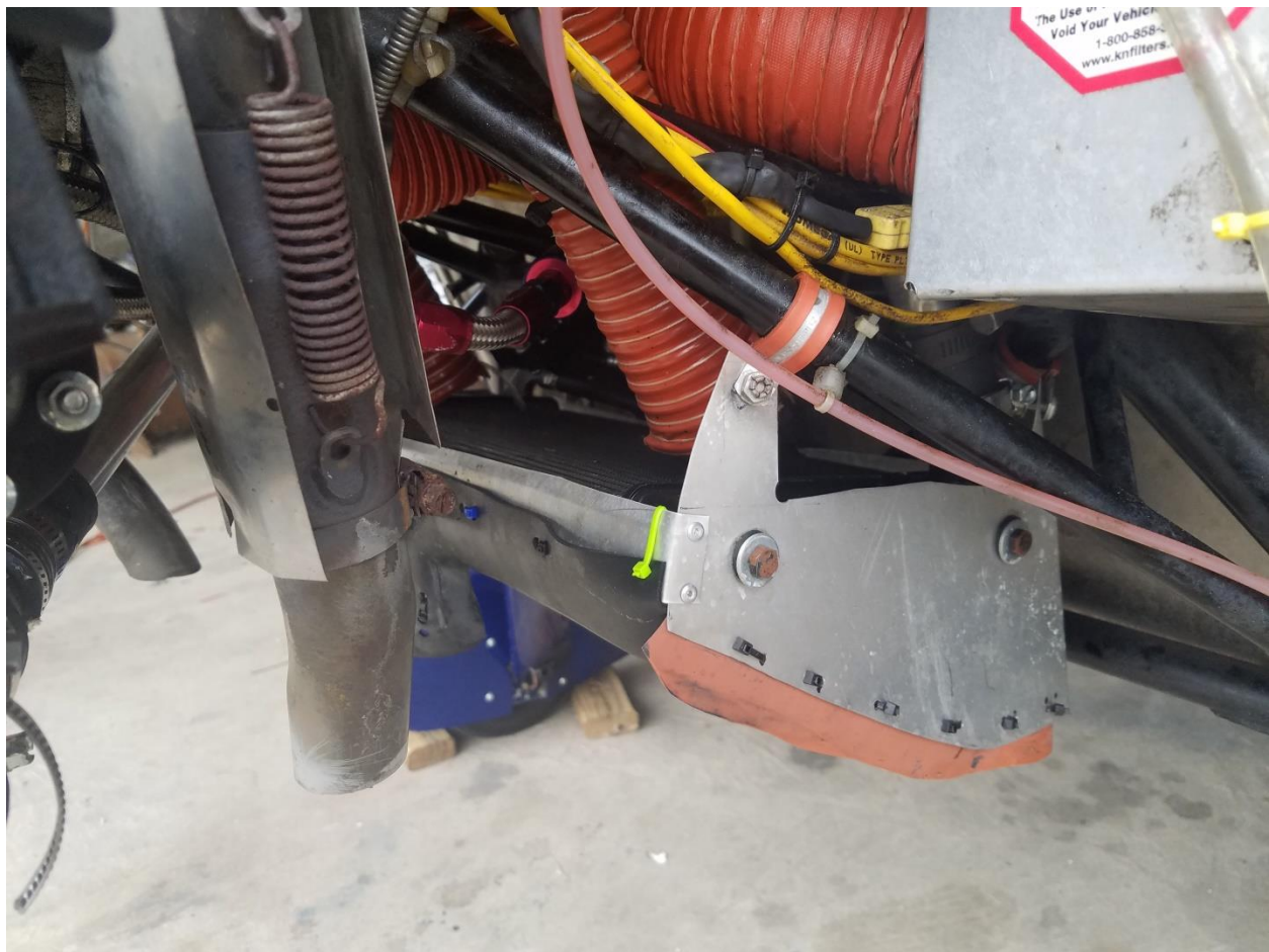
Figure 1. Location of the radiator. Suspended from the engine mount, baffled to the cowl wall
