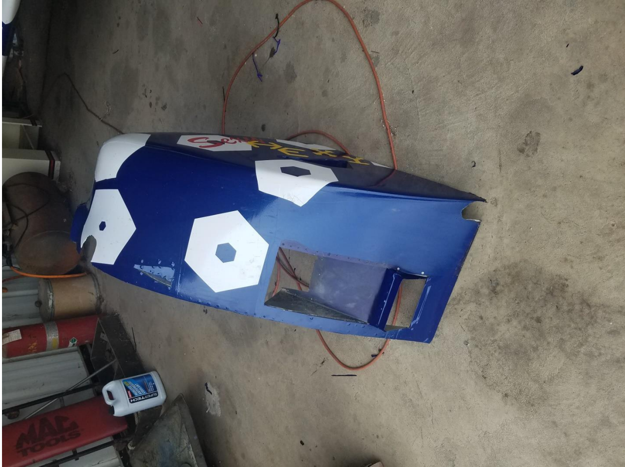
Figure 4. Modified cowl. Note the original cowl opening, and the new cowl opening with the air dam. Also note the new oil cooler NACA duct. One on each side.
