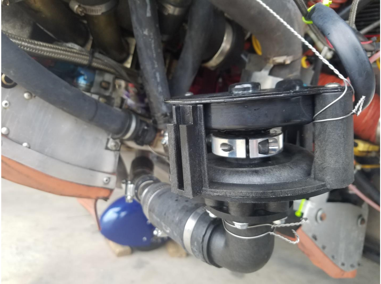
Figure 3. Clamp on Seal Boss. Poor quality control. The pump will come off soon enough and be replaced with something of better quality.
